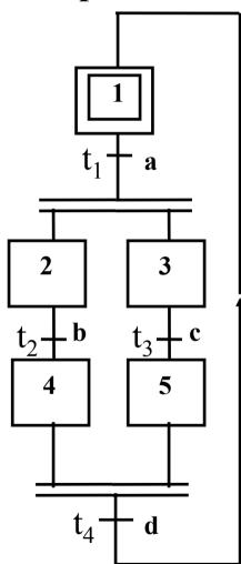
$$Dq = 0 \qquad D = \begin{bmatrix} -1 & 0 & 0 & 1 \\ 1 & -1 & 0 & 0 \\ 1 & 0 & -1 & 0 \\ 0 & 1 & 0 & -1 \\ 0 & 0 & 1 & -1 \end{bmatrix} q = \begin{bmatrix} \sigma_1 \\ \sigma_2 \\ \sigma_3 \\ \sigma_4 \end{bmatrix}$$
