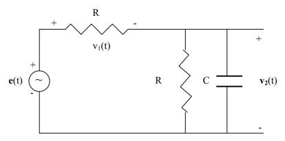
In the circuit depicted in the previous figure,  $\mathbf{e}(t)$  is a telegraphic signal that can assume the values 1 V e -1 V, being both equi-provable. The duration of each pulse is described by a Poisson process.
