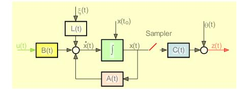
STATISTICAL INFORMATION (4)  $E\{x(t_0)\} = \bar{x}_0; cov[x(t_0); x(t_0)] = \Sigma_0$ (5)  $E\{\xi(t)\} = 0; cov[\xi(t); \xi(\tau)] = \Xi(t)\delta(t - \tau)$ (6)  $E\{\theta(t_k)\} = 0; cov[\theta(t_k); \theta(t_j)] = \Theta(t_k)\delta_{t_kt_j}$ • All variables are assumed gaussian •  $x(t_0), \xi(t), \theta(t_k)$  independent
