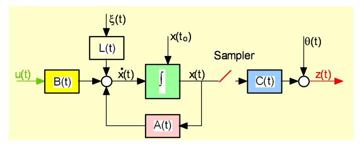
The discrete - time measurements are visualized using a SAMPLER that closes at discrete - instants of time t<sub>1</sub>, t<sub>2</sub>, ..., t<sub>k</sub>, t<sub>k+1</sub>, ...
