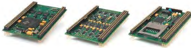
Figure 2.10: Core processing unit. From left to right: D.Module.C6713, D.Module.ADDA16, D.Module.91C111.
